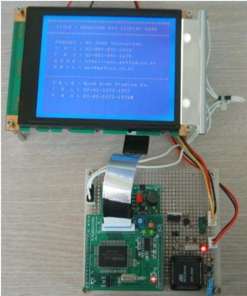
Test LCD Module Module(UG-32F03-BCBN8-C)
